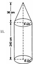
Let us suppose that r denotes the radius of the cylinder = 8 cm. Suppose R denotes the radius of the cone = 8 cm. Let h be the height of the cylinder = 240cm. Suppose H is the height of the cone = 36 cm. Total volume of the iron = volume of the cylinder + volume of the cone  $=\pi r^2h+rac{1}{3}\pi R^2H=\pi r^2\left(h+rac{1}{3}H
